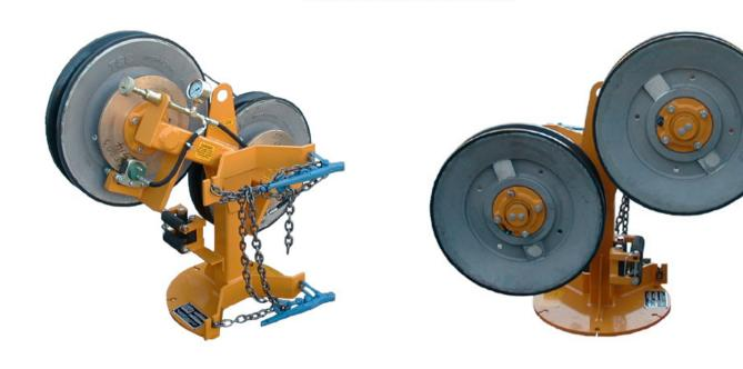
The 3505 tensioner module is designed to provide higher conductor stringing tension than possible from braked reel stands. It can be pole mounted, truck or trailer base plate mounted and is to be used in conjunction with a suitable conductor reel let-off stand.
